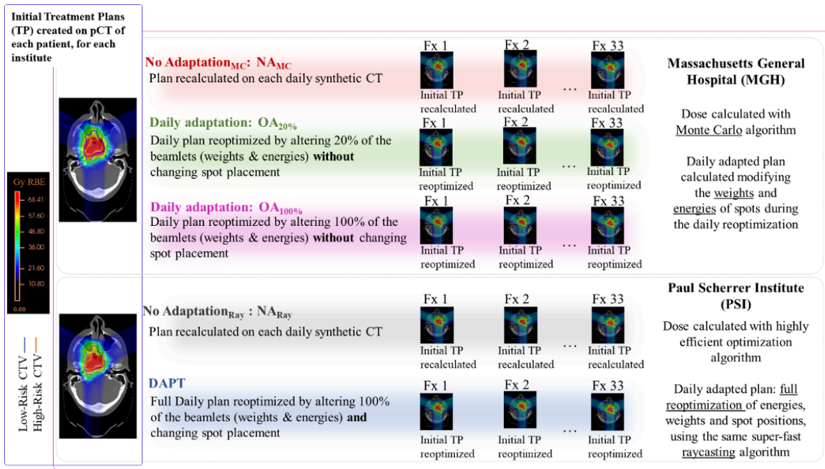
Figure 1. The figure shows the simulated workflows. Each patient has a no-adaptation workflow where the daily plan is recalculated on the daily image. In addition, for each patient, a full reoptimization (DAPT) was simulated, and two other adaptation strategies where 20% and 100% of the beamlets were changed without changing the spot placement.
